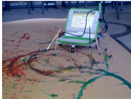
Figure 14. Floor turtle 2014-style (by Cecilia Vilaró). The Butia robot powered by TurtleBots. Through the plugin mechanism, Turtle Blocks talks to an arduino that controls sensors and motors, including an actuator to implement “pen up” and “pen down” commands.
