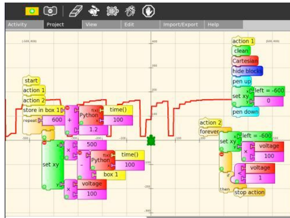
Figure 8. Measuring gravitational acceleration. Shown above is a triggerable oscilloscope with calibrated time base. “Action 1” clears the screen and draws the scale, the program waits in “action 2” until triggered by the first switch. The graphing then starts. Switches were placed at 20 cm, 60 cm, 100 cm, 140 cm, and 180 cm along a ramp of length 180 cm and height 25 cm.
